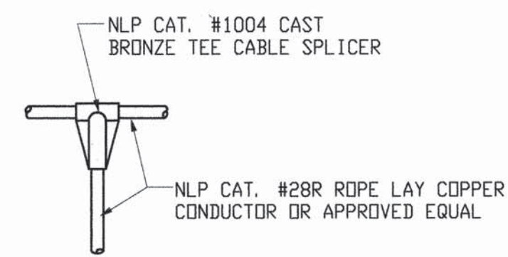
TYPICAL TEE CABLE SPLICE NOT TO SCALE
