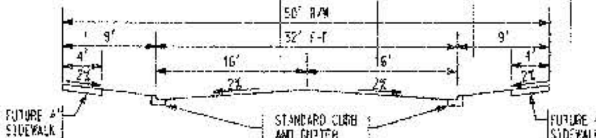
TYPICAL STREET SECTION LOCAL RESIDENTIAL NO SCALE
