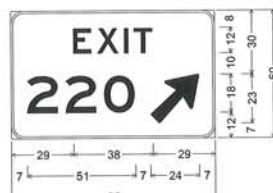
Sign 0705; 6" Radius, 1" Border, White on Green; [EXIT] E; [220] E; Arrow 13.33UC-12CAP-A - 29° 45';
