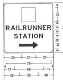
Sign 0910; 6" Radius, 1" Border, White on Green; Railrunner Logo; [RAILRUNNER] E; [STATION] E; Arrow 8" Type D4 - 32° 0';
