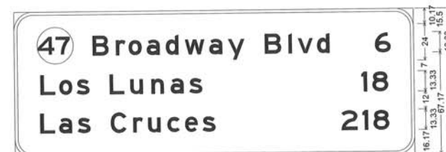
Sign 1202; 12.00" Radius, 2.00" Border, White on Green; 47 Shield; [Broadway Blvd] E; [6] E; [Los Lunas] E; [18] E; [Las Cruces] E; [218] E;
