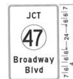
Signs 1702; 1704; 3.0" Radius, 1.0" Border, White on Green; [JCT] D; Shield; [Broadway] D; [Blvd] D;
