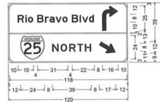
Sign 1925; 6" Radius, 1" Border, White on Green; [Rio] E 50% spacing; [Bravo] E 50% spacing; [Blvd] E 50% spacing; 90 Deg Advance Turn Arrow Custom 16" X 25°; [NORTH] E: Arrow 8" Type D2 - 18" 330°;
