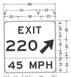
Sign 1002; 6" Radius, 1" Border, White on Green; [EXIT] E; [220] E; Arrow 13.33UC-12CAP-A - 29° 45'; 6" Radius, 1" Border, Black on Yellow; [45 MPH] E;
