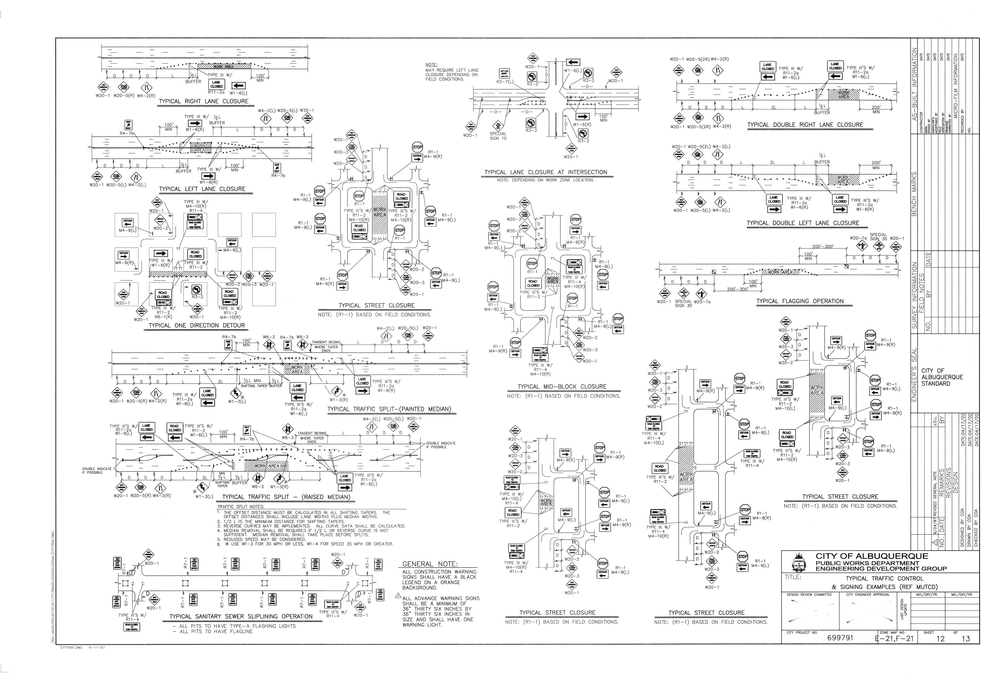
2. CONTRACTOR SHALL AT THE TIME OF PERMIT REQUEST, SUBMIT FOR APPROVAL BY CONSTRUCTION COORDINATION, A TRAFFIC CONTROL PLAN DETAILING ALL EXISTING TOPOGRAPHY SUCH AS LANE WIDTHS, DRIVEWAYS, AND BUSINESS/RESIDENTIAL ACCESSES. THE TRAFFIC CONTROL PLAN SHALL INCLUDE ALL PHASES OF WORK AND SCHEDULES INVOLVED IN THE CONSTRUCTION PROJECT. ANY SEPERATE PHASES OF A CONSTRUCTION PROJECT SHALL BE GIVEN AN INDIVIDUAL PERMIT EACH. BLANKET PERMITS WILL NOT BE ISSUED.
