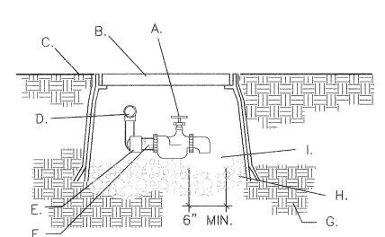
MANUAL DRAIN (SEE IRRIGATION LEGEND) BROOKS PRODUCTS INC. 1419-18 VALVE BOX WITH BOLT DOWN COVER WITH ONE 8" EXTENSION FINISH GRADE MAINLINE OR LATERAL MAIN
