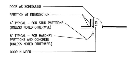
WALLS AND PARTITIONS ARE DIMENSIONED FROM FACE OF MASONRY OR STUDS UNLESS NOTED OTHERWISE.
