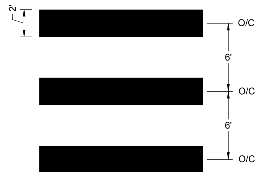
CROSSWALK BAR SPACING DETAIL NOT TO SCALE
