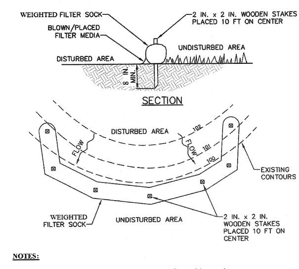
Weighted filter socks may be used on impervious surfaces without stakes.
