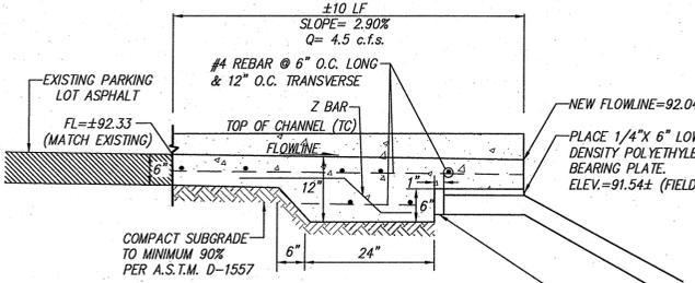
PLACE 1" POLYETHYLENE FOAM FILLERS AS SHOWN. PLASTIZONE OR APPROVED EQUAL DO NOT ANCHOR WITH NAILS OR BONDING AGENT. KEEP IN PLACE WITH FRESH CONCRETE WHEN POURING UPSTREAM SECTION. DO NOT ALLOW FRESH CONCRETE BETWEEN FILLER AND PREVIOUS CONCRETE.
