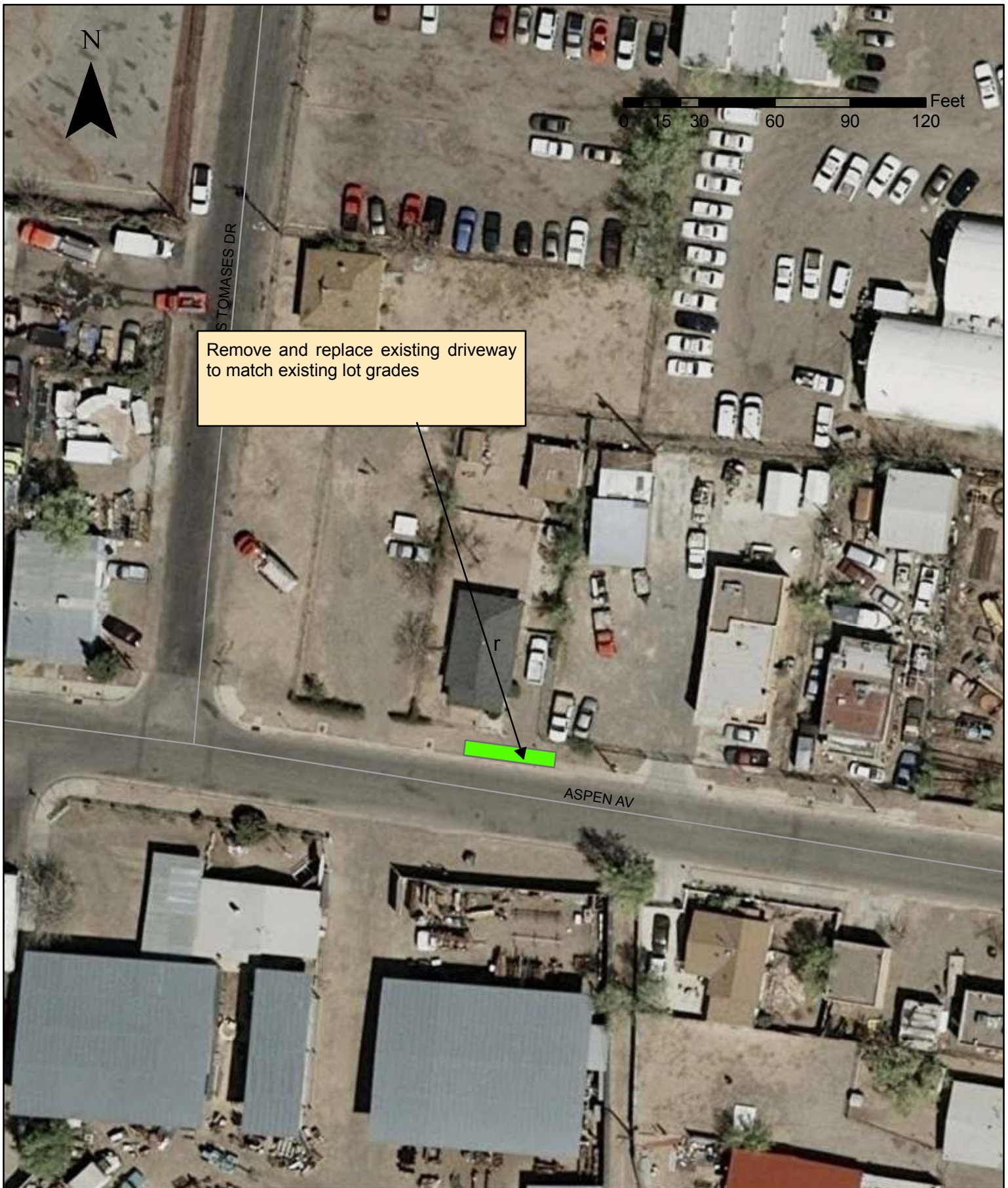
Dirveway reconstruction 621 Aspen Ave.
