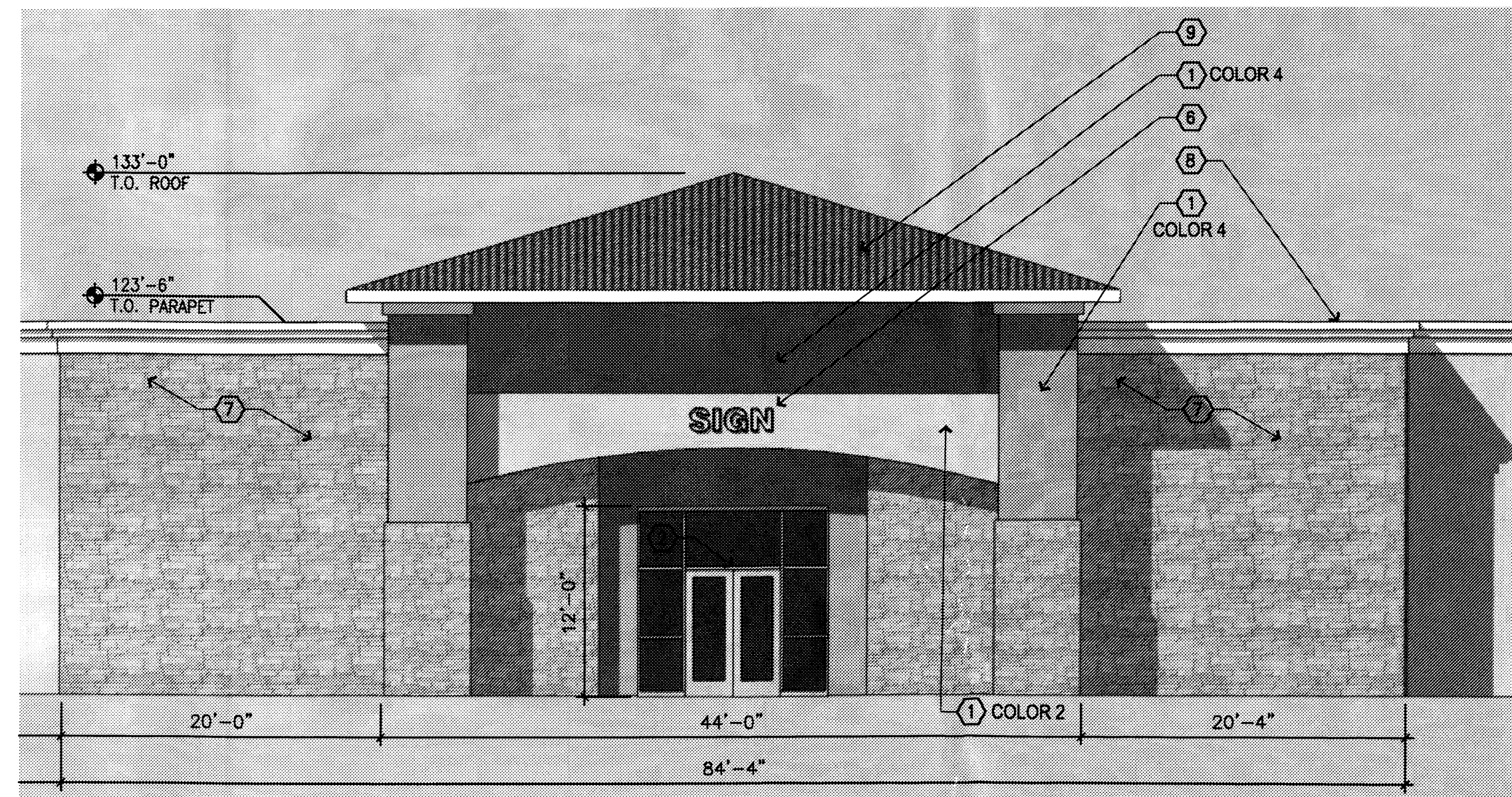
2 BUILDING ELEVATION - PARTIAL NORTH 1/8" = 1'-0"
