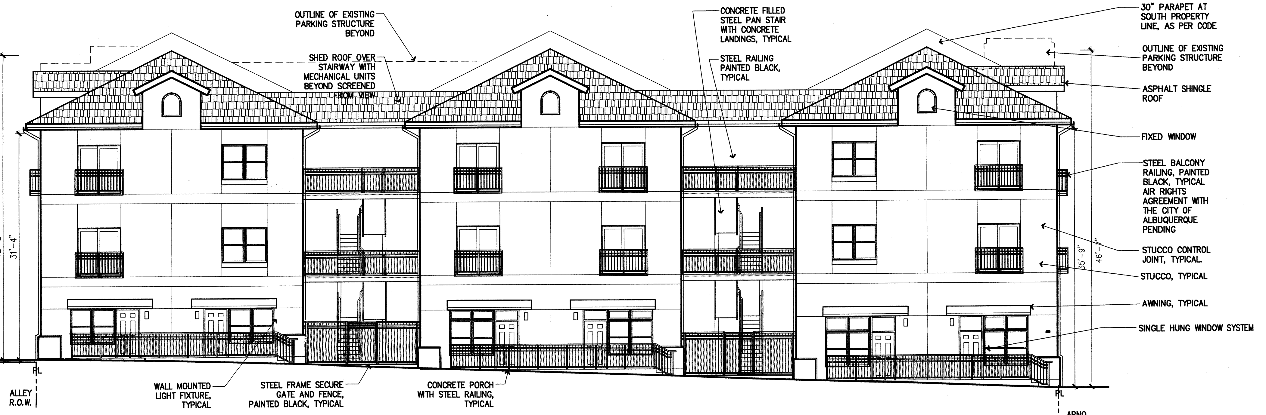
4 COPPER NORTH ELEVATION 1/8" = 1'-0"
