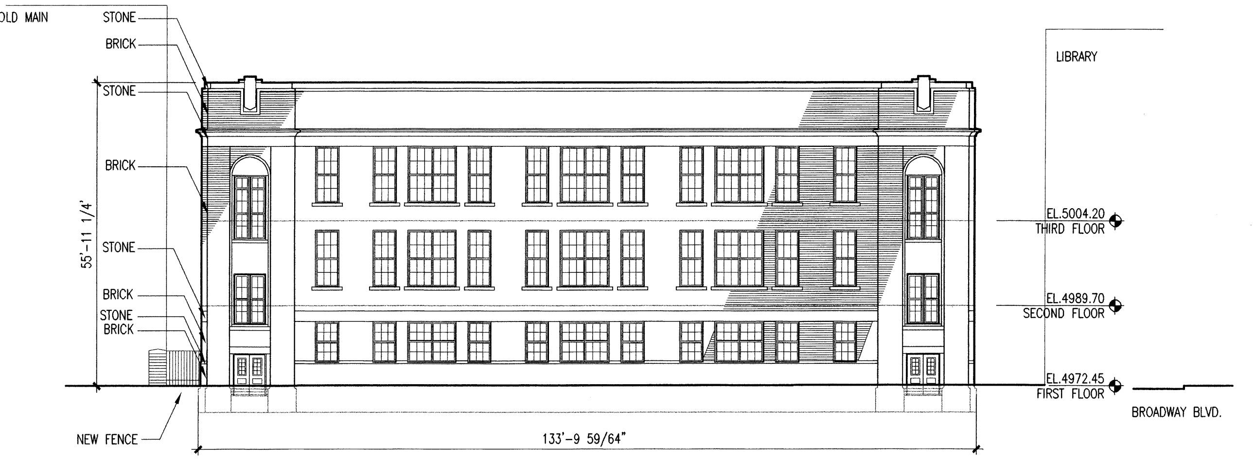
4 Classroom - Existing East Elevation 1/16"=1'-0"
