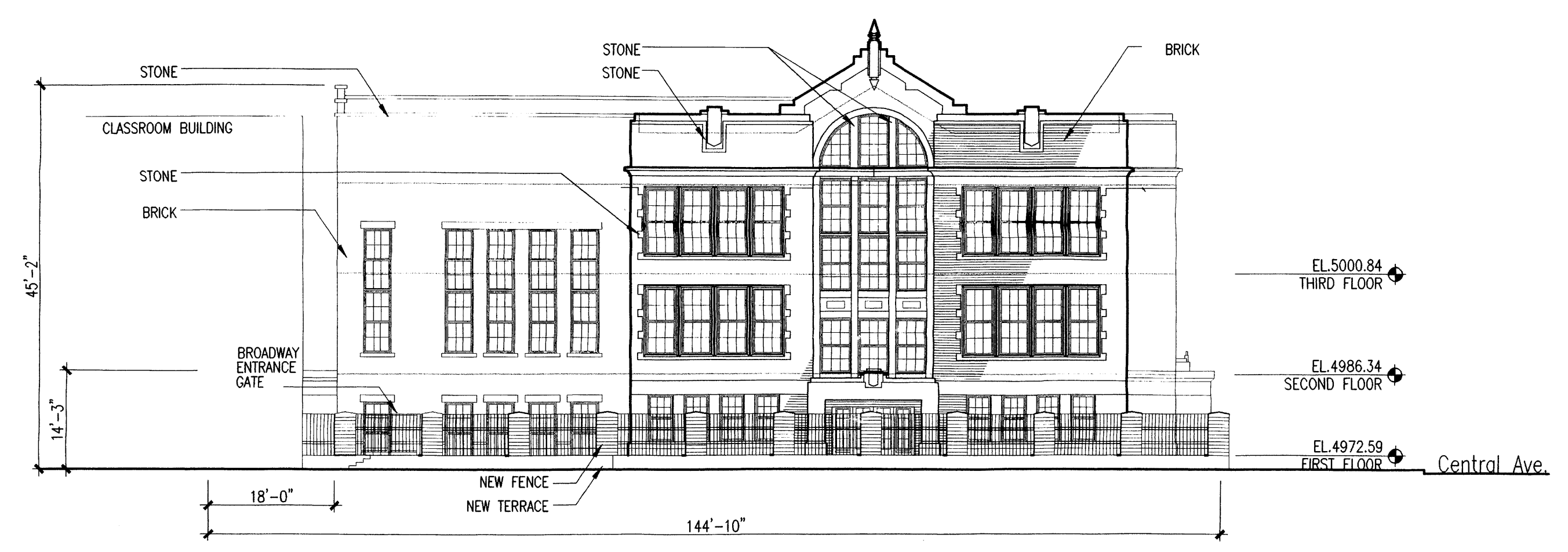
6 Old Main - Existing West Elevation 1/16"=1'-0"
