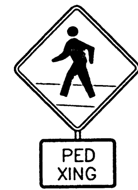
PEDESTRIAN CROSSING SIGN SCALE: NTS BLACK LEGEND ON YELLOW BACKGROUND (W11A-2) (W11A-2P)
