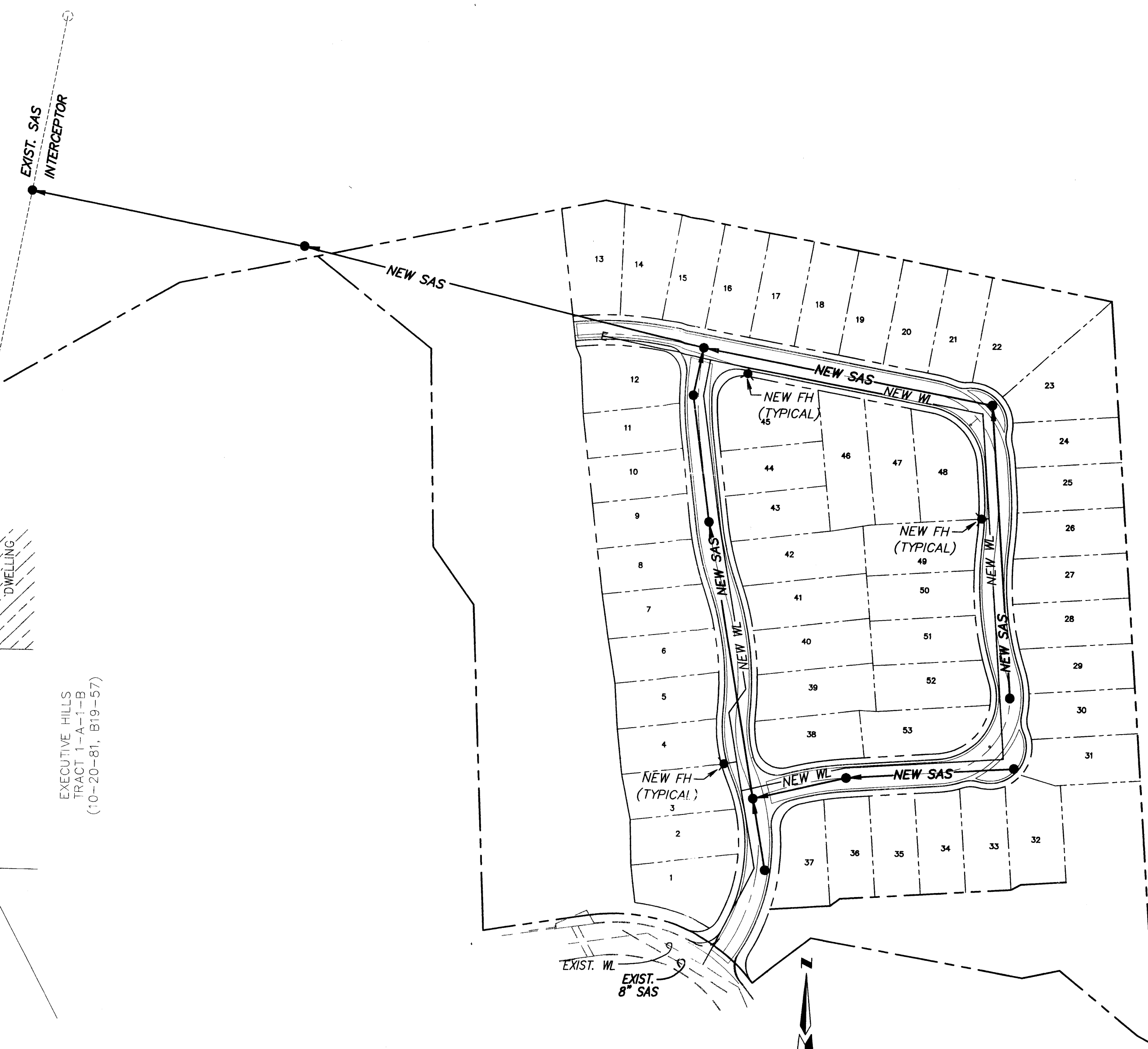
NEW UTILITY LAYOUT (UTILITY DEVELOPMENT) SCALE: 1" = 100'
