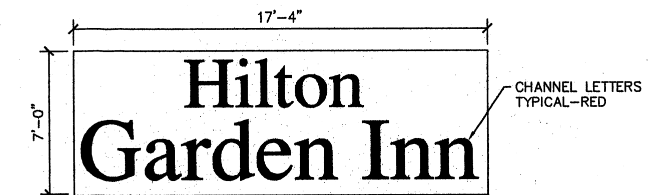
BUILDING MOUNTED SIGN SCALE: 1/4"=1'-0"
