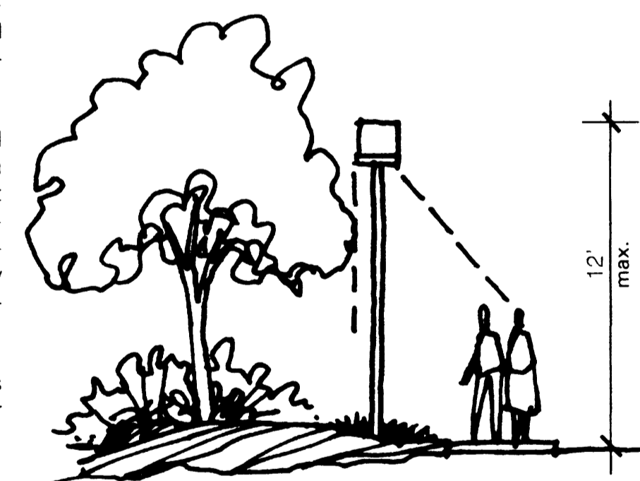
Shielded source site lighting
