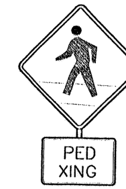
BLACK LEGEND ON YELLOW BACKGROUND (W11A-2) (W11A-2P) PEDESTRIAN CROSSING SIGN SCALE: NTS
