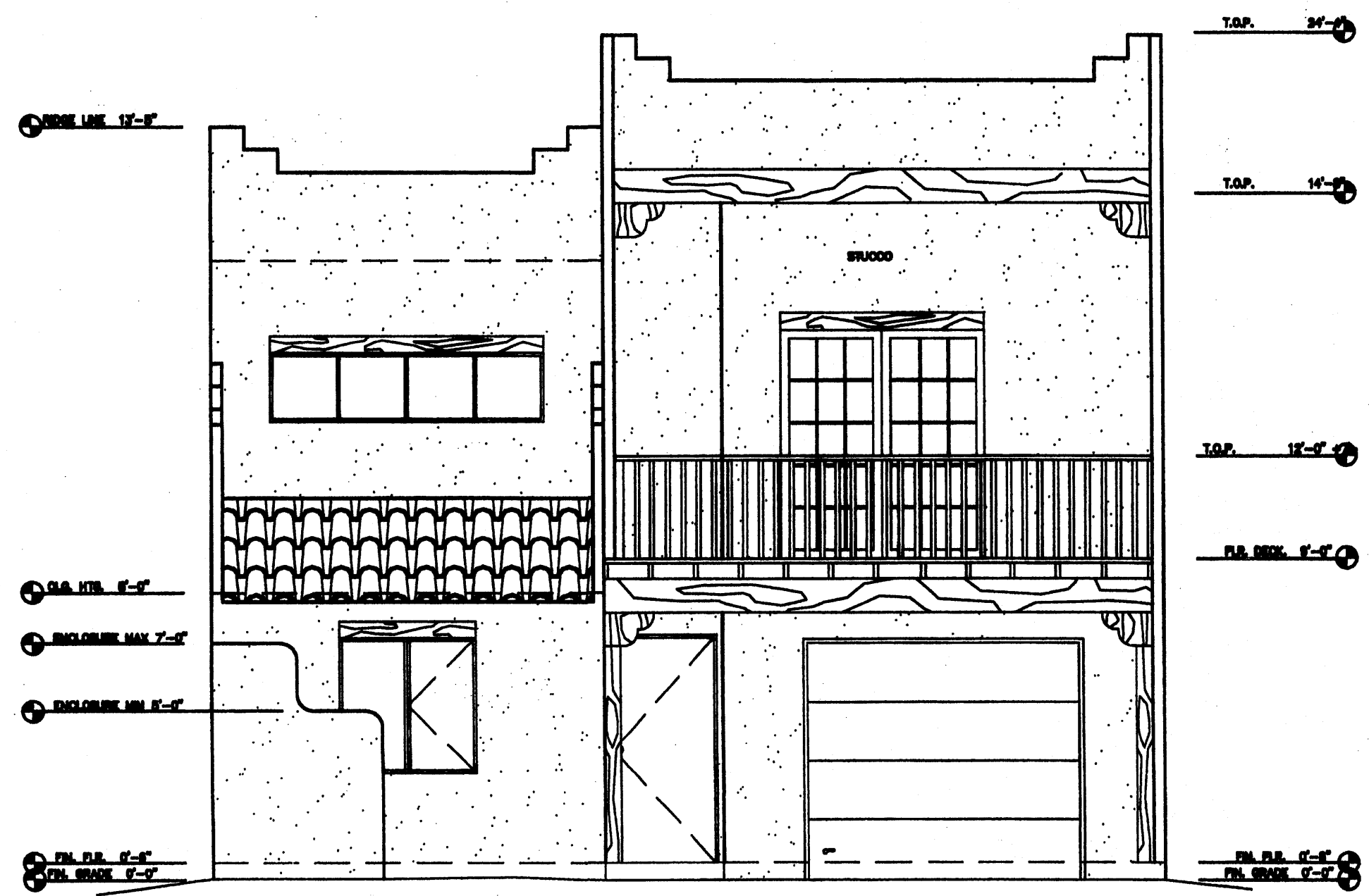
FRONT ELEVATION SCALE: 1/4" = 1'-0"
