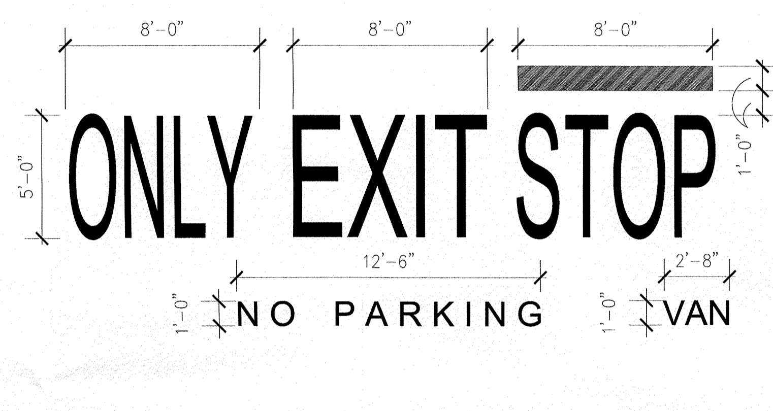
7 MARKING DETAILS F4.1 1/4" = 1' - 0" NOTES: OVERALL DIMENSIONS TYP. FOR SINGLE WORD PAVEMENT MARKINGS. USE WHITE EVER-BRITE (CALAPHOTE INC.) OR APPROVED EQUAL THERMOPLASTIC.
