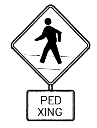
BLACK LEGEND ON YELLOW BACKGROUND (W11A-2) (W11A-2P) PEDESTRIAN CROSSING SIGN SCALE: NTS
