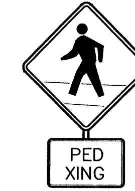
BLACK LEGEND ON YELLOW BACKGROUND (W11A-2) (W11A-2P) PEDESTRIAN CROSSING SIGN SCALE: NTS
