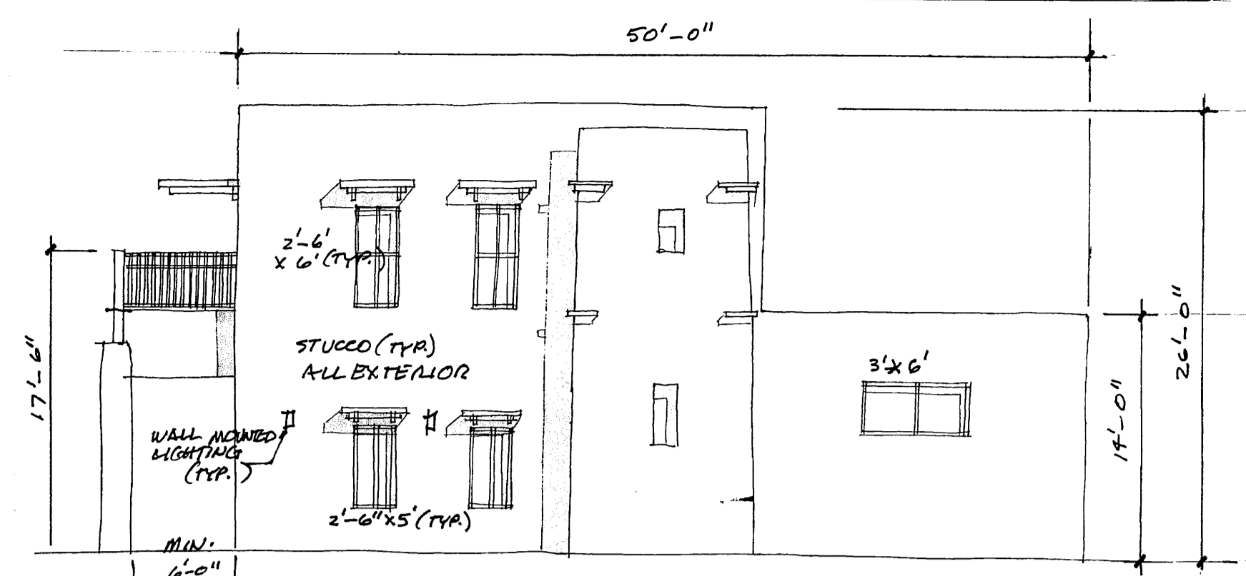
SOUTH ELEVATION BUILDING 'D' 1/8" = 1'-0"
