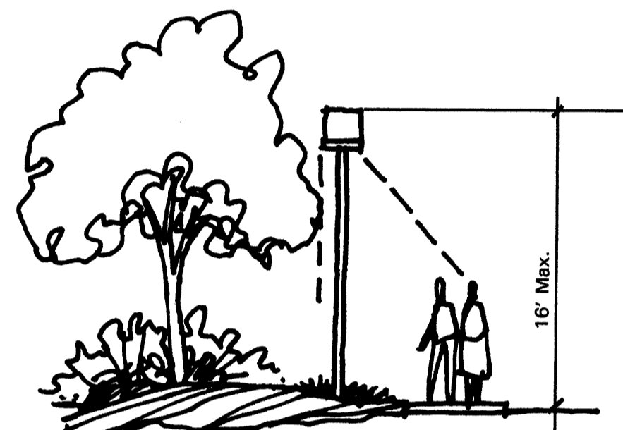
LIGHTING - should be shielded source, with the height kept to a minimum necessary to meet safety standards
