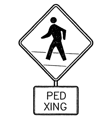
PEDESTRIAN CROSSING SIGN BLACK LEGEND ON YELLOW BACKGROUND (W11A-2) (W11A-2P) SCALE: NTS
