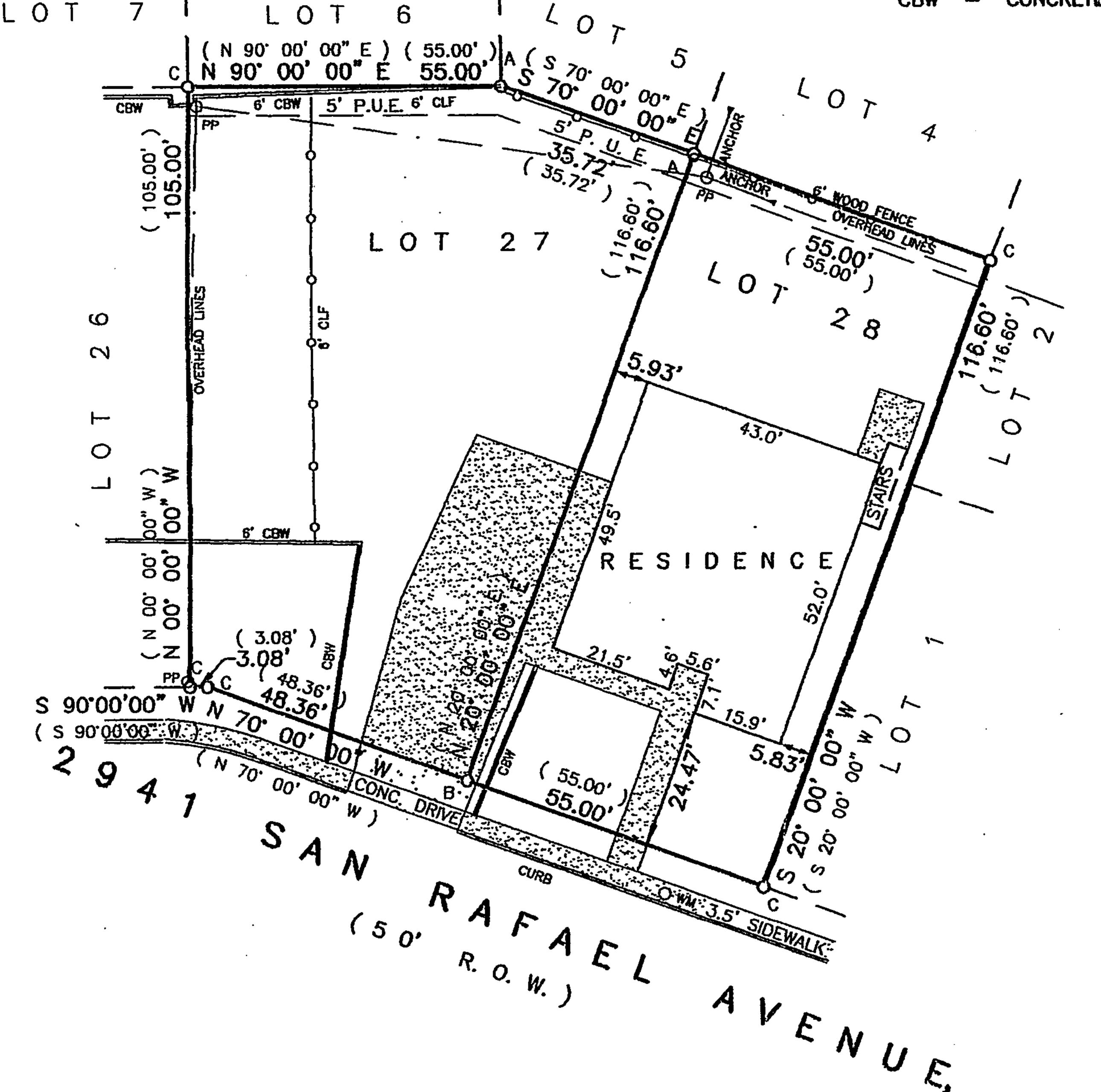
BEARINGS AND DISTANCES SHOWN ARE FIELD MEASURED. BEARINGS AND DISTANCES IN PARFNTHESIS ARE RECORD. ALL FOUND AND ACCEPTED MONUMENTS TAGGED "PS 14269".
