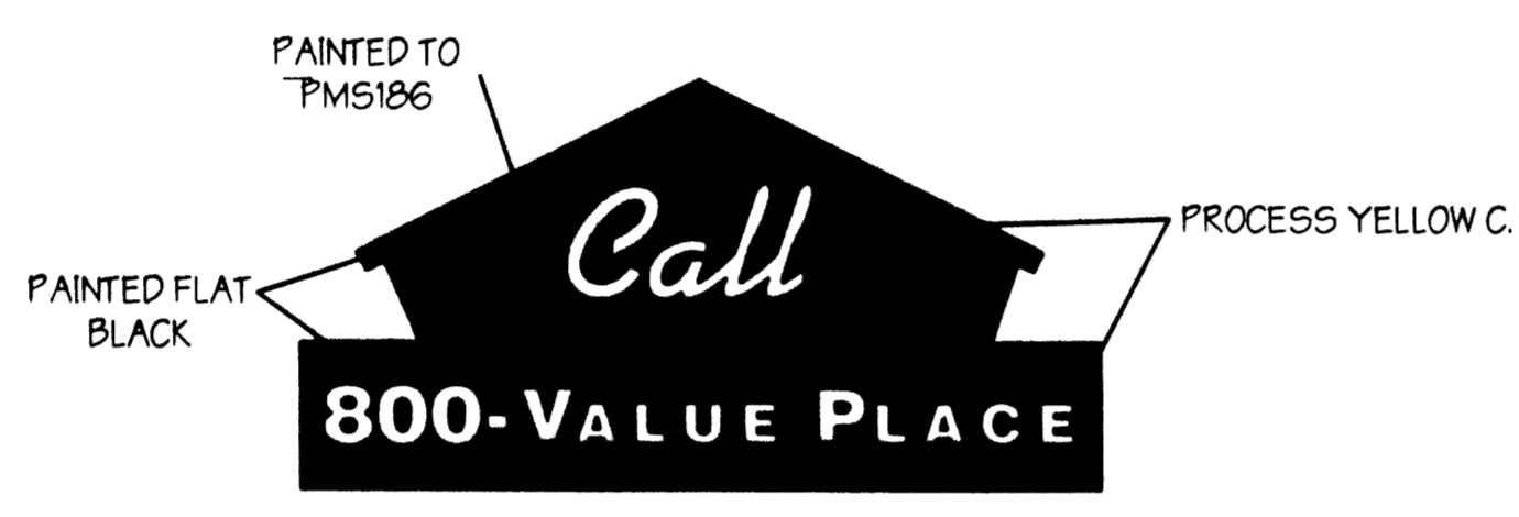
NORTH END ELEVATION WITH WALL SIGN 3/32" = 1'
