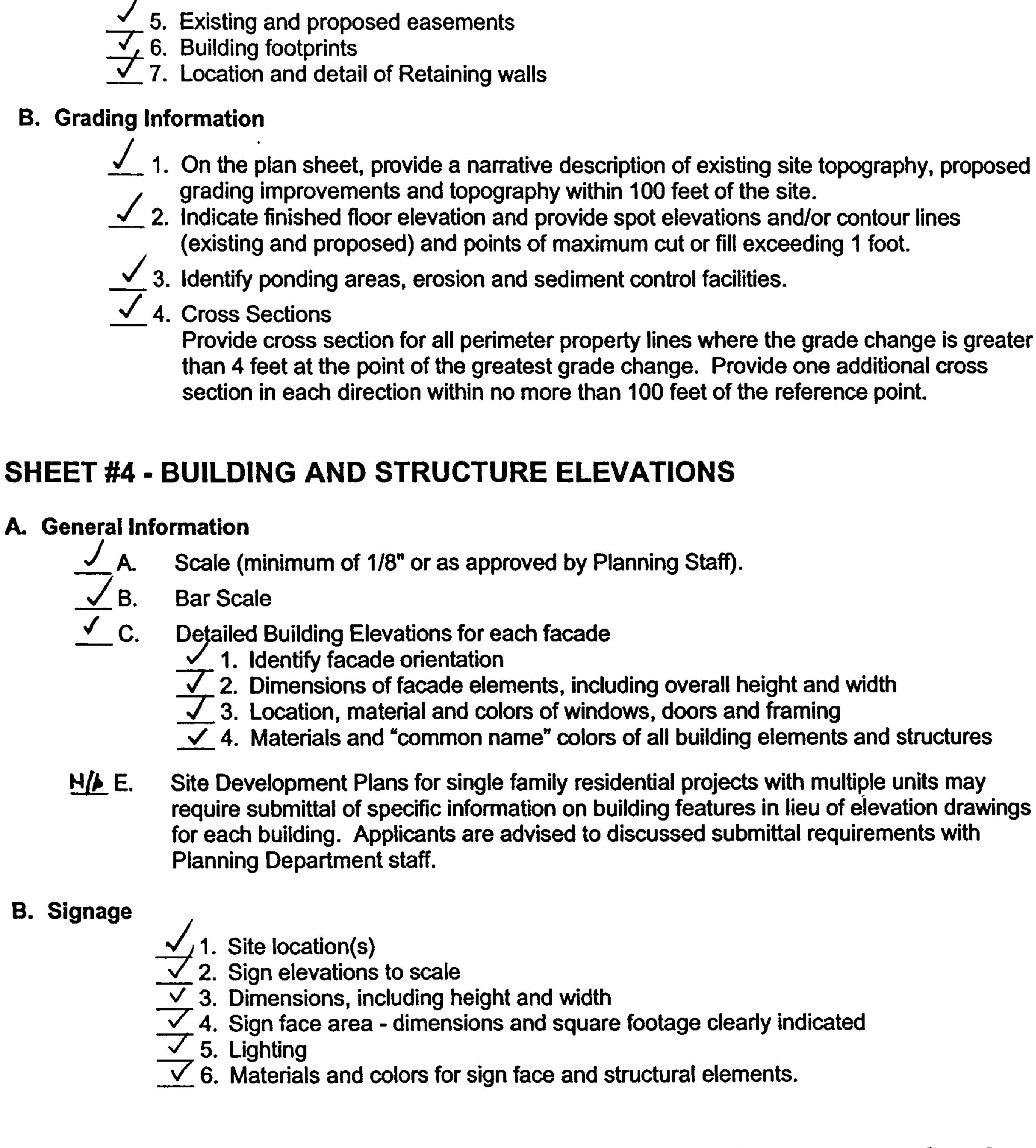
Applicants should make sure that the submitted site development plan drawings are accurate and complete, and that items specified in this checklist have been clearly indicated on the plan drawings as required.
