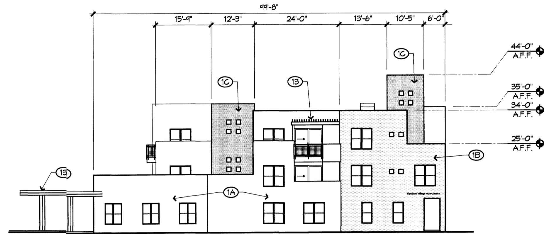
B1 WEST ELEVATION BUILDING A
