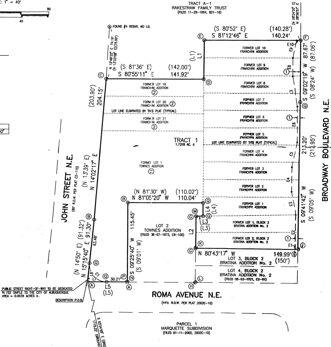
NEW MEXICO CENTRAL ZONE-NAD 1927 A.C.S. STA. "6-K14(R)" X=382,162.22 Y=1,485,941.10 COMBINED FACTOR=0.99967824 DELTA ALPHA=-IX013/35" ELEVATION=4968 765' (NGVD 29)
