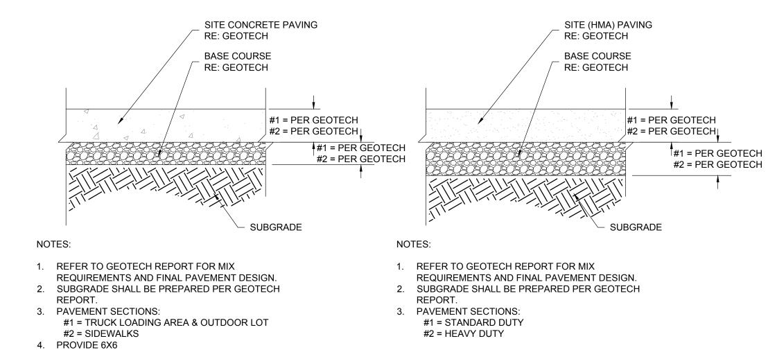
5. CONCRETE SHALL BE 4500 PSI MIN OR GREATER IF REQUIRED BY GEOTECH.
