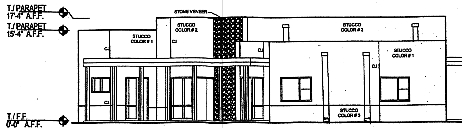
A3 Building F - South Exterior Elevation 1/8" - 1'-0"
