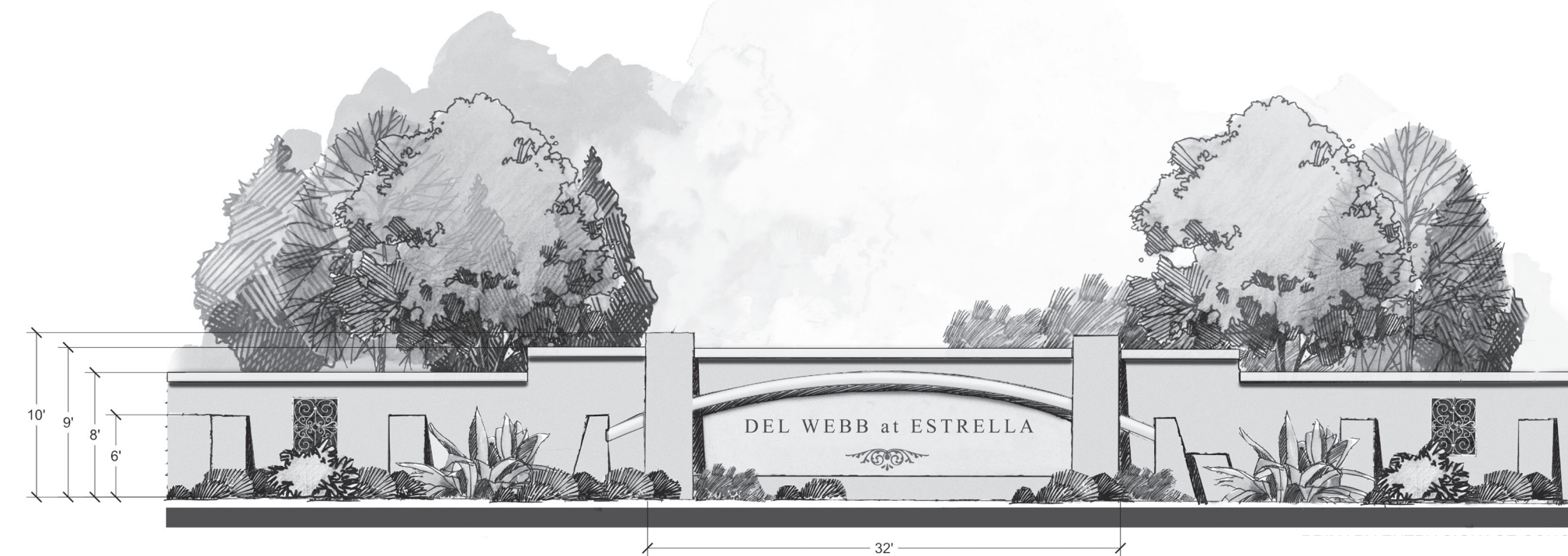
M. ILLUSTRATIVE SECONDARY COMMUNITY ENTRY - B Max. Height: 6 feet. Max. Length: 12 feet. Max. Sign face: 35 SF.
