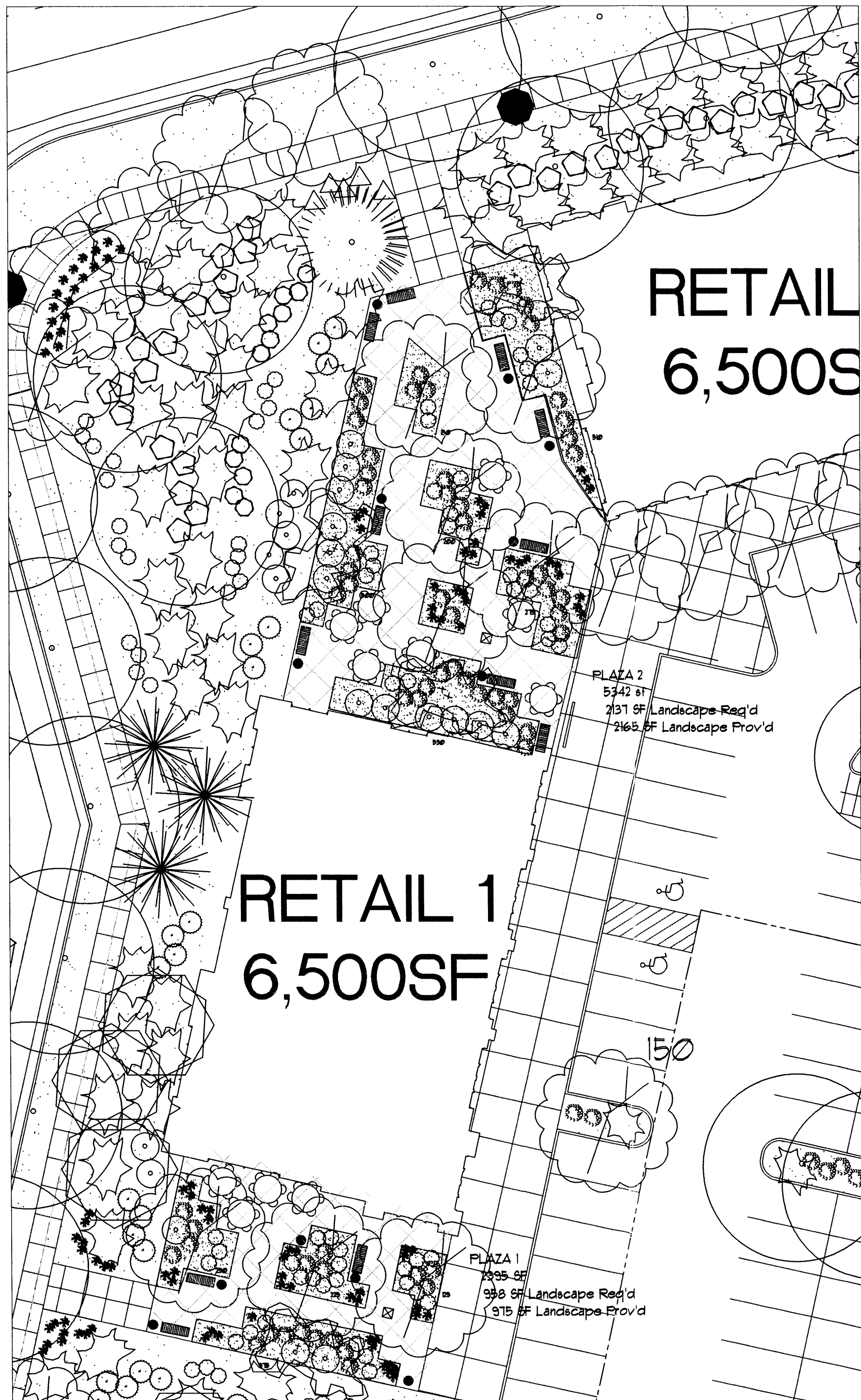
PLAZA 1 AND 2, DETAIL LANDSCAPE BEDS TO BE 80% LIVE GROUND COVER AT MATURITY.
