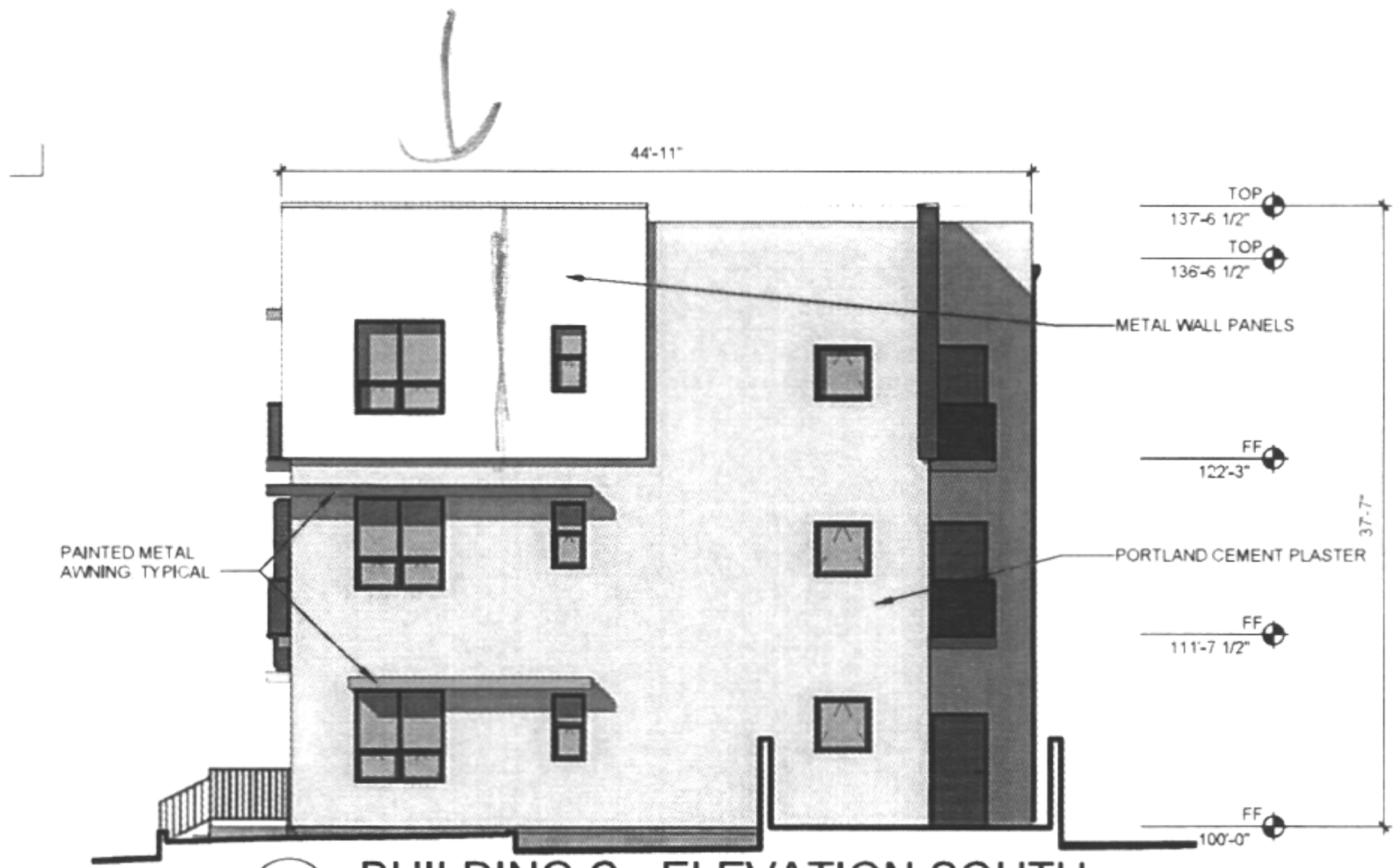
5 BUILDING C - ELEVATION SOUTH 1/8" = 1'-0"
