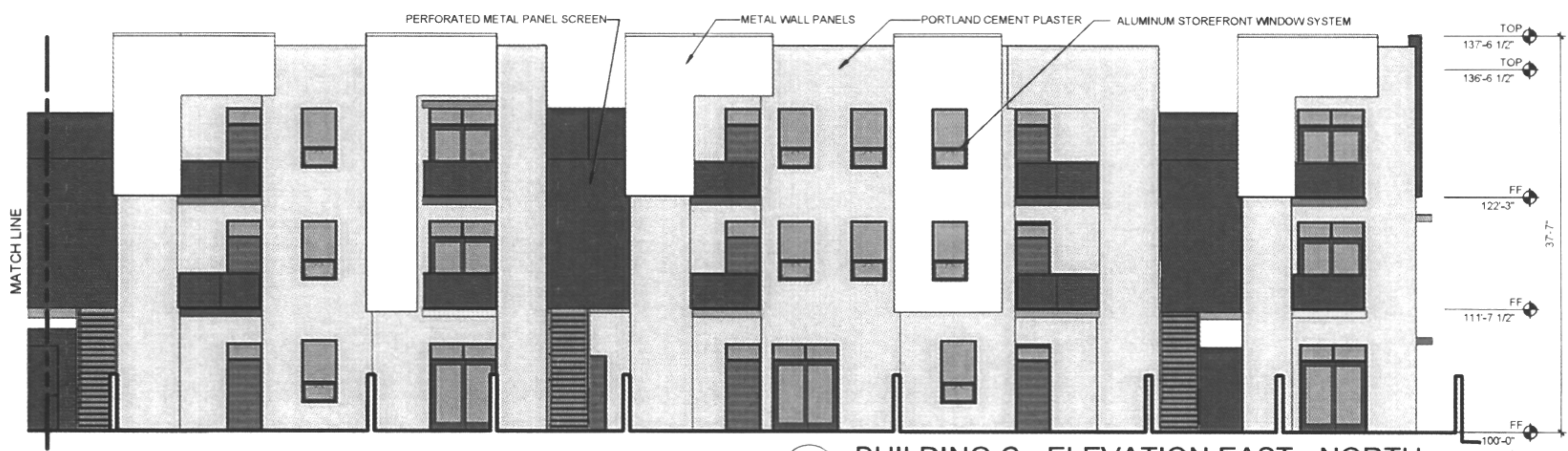
6 BUILDING C - ELEVATION EAST - NORTH 1/8" = 1'-0"
