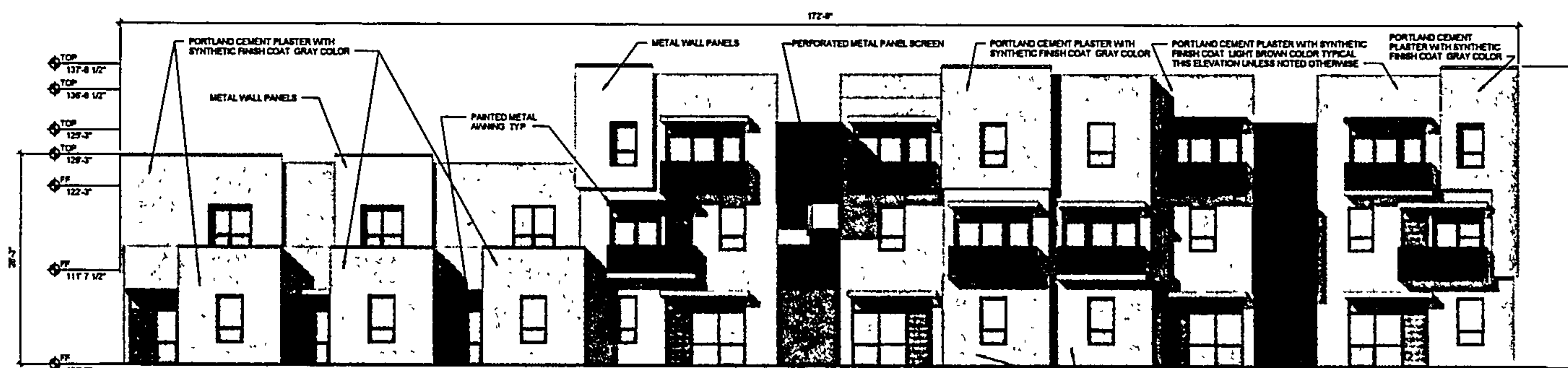
1 BUILDING D - ELEVATION SOUTH 1/8" = 1'-0"
