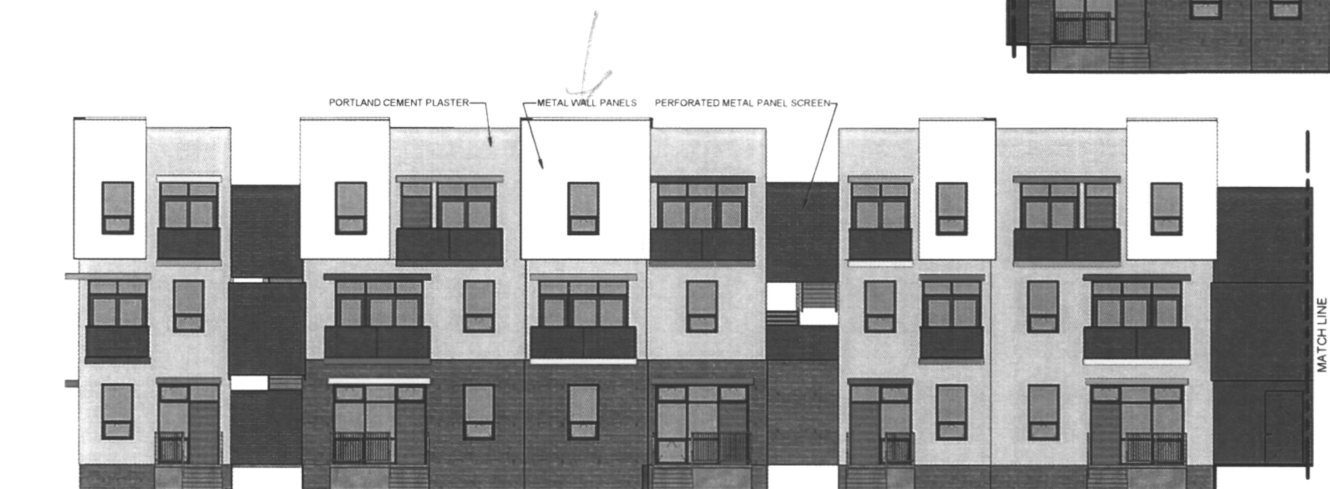
1 BUILDING C - ELEVATION WEST - NORTH 1/8" = 1'-0"
