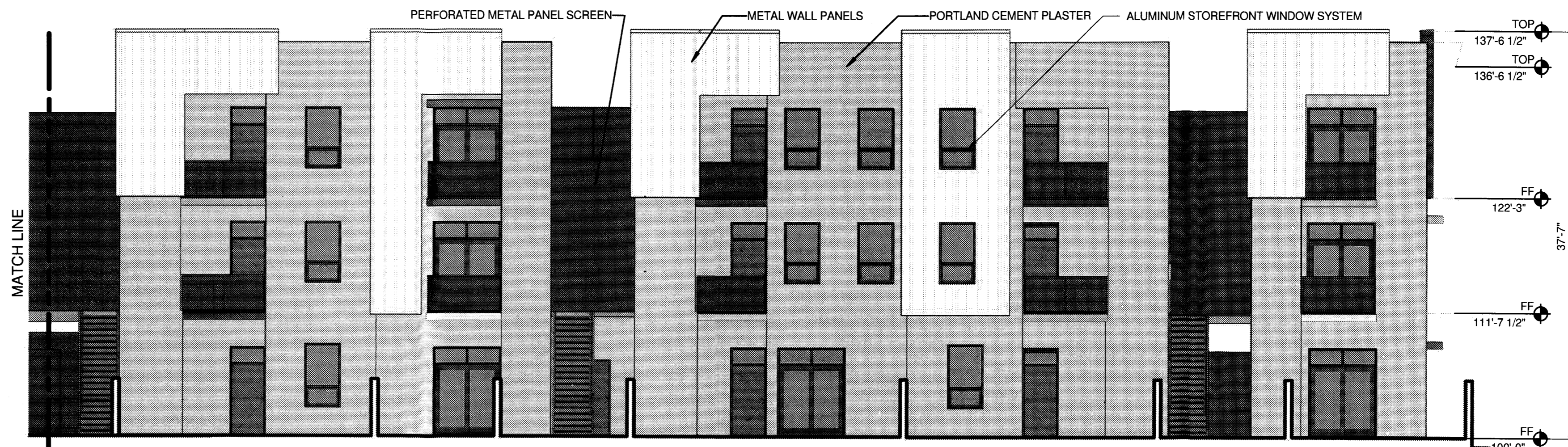
6 BUILDING C - ELEVATION EAST - NORTH 1/8" = 1'-0"
