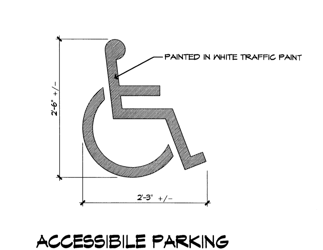
8 ACCESSIBLE PARKING PAVEMENT MARKING 1" = 1'-0"
