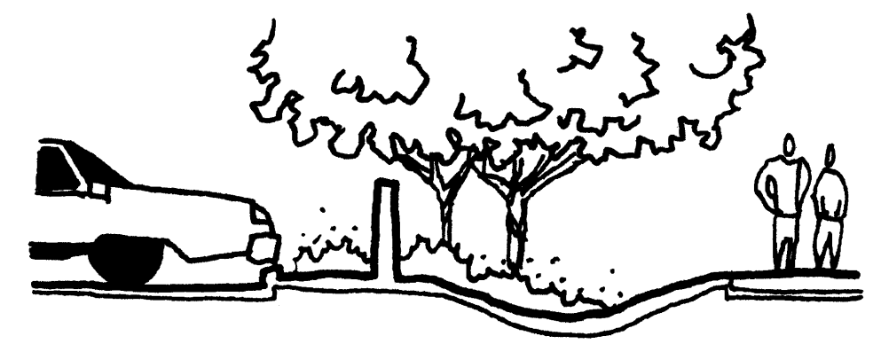
Low-wall used to screen parking areas from roadways
