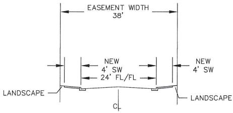
SIGNAL POINTE - NORTH/SOUTH PROPOSED CROSS-SECTION
