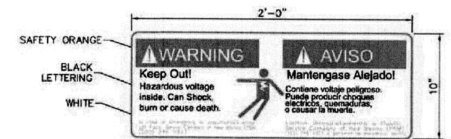
SAFETY WARNING SIGN (No Scale) FOR SAFETY PURPOSES AS REQUIRED BY NESC.
