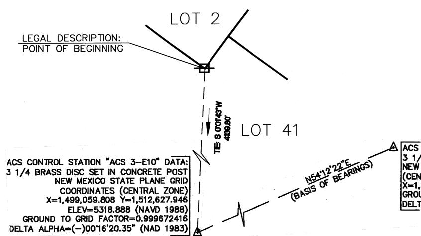
ACS CONTROL STATION "ACS 13-D10" DATA: 3 1/4 BRASS DISC SET FLUSH IN LAVA ROCK NEW MEXICO STATE PLANE GRID COORDINATES (CENTRAL ZONE) X=1,501,318.610 Y=1,514,256.686 GROUND TO GRID FACTOR=0.999672421 DELTA ALPHA=(-)0016'04.84" (NAD 1983)
