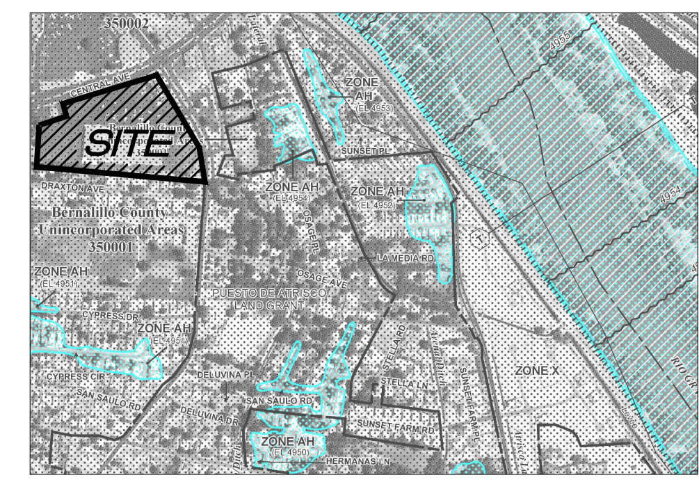
FIRM MAP 35001C0333H Per FIRM Map 35001C0333H, dated August 16, 2012, the site is located in the 0.2% chance Annual Floodplain with Average Depth of less than 1 foot.
