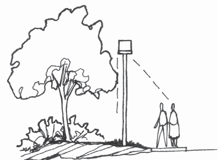
LIGHTING - should be shielded source, with the height kept to a minimum necessary to meet safety standards
