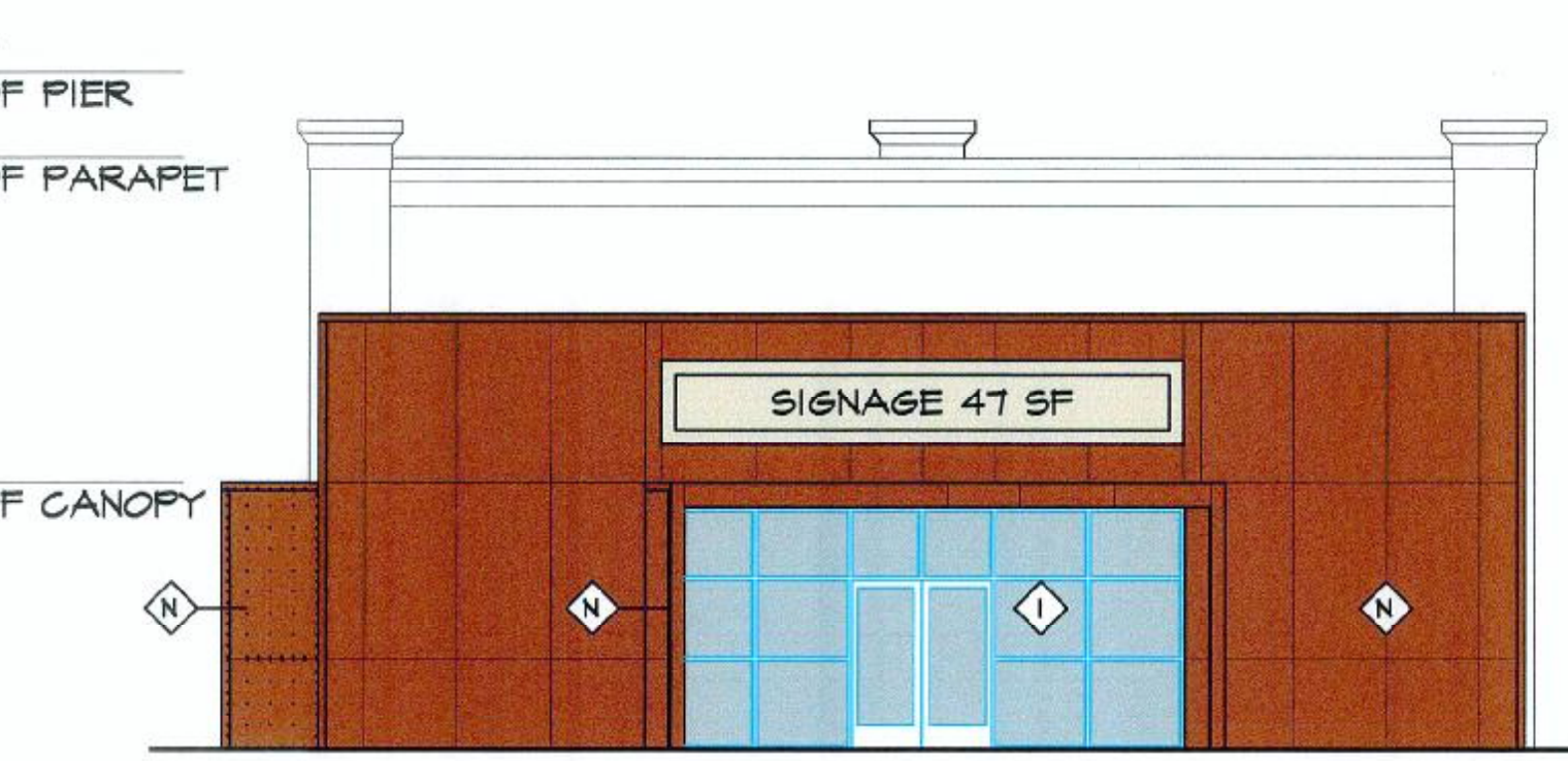
SOUTH ELEVATION SIGNAGE: 47 SF OF 935 SF FACADE = 5.03% 1/8" = 1' - 0" 0 8' 16'
