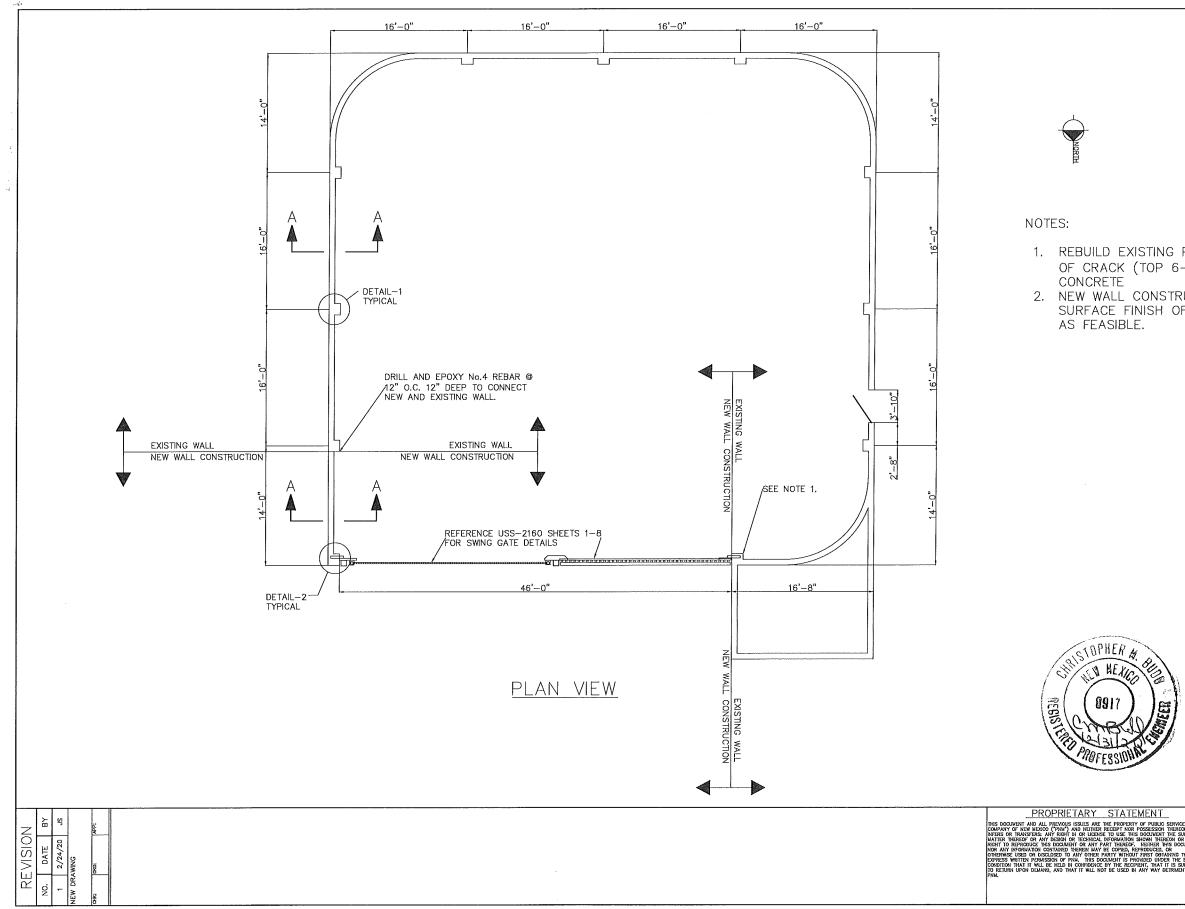
REBUILD EXISTING PILASTER FROM TOP TO THE END OF CRACK (TOP 6-7 COURSES). FILL WITH CONCRETE
