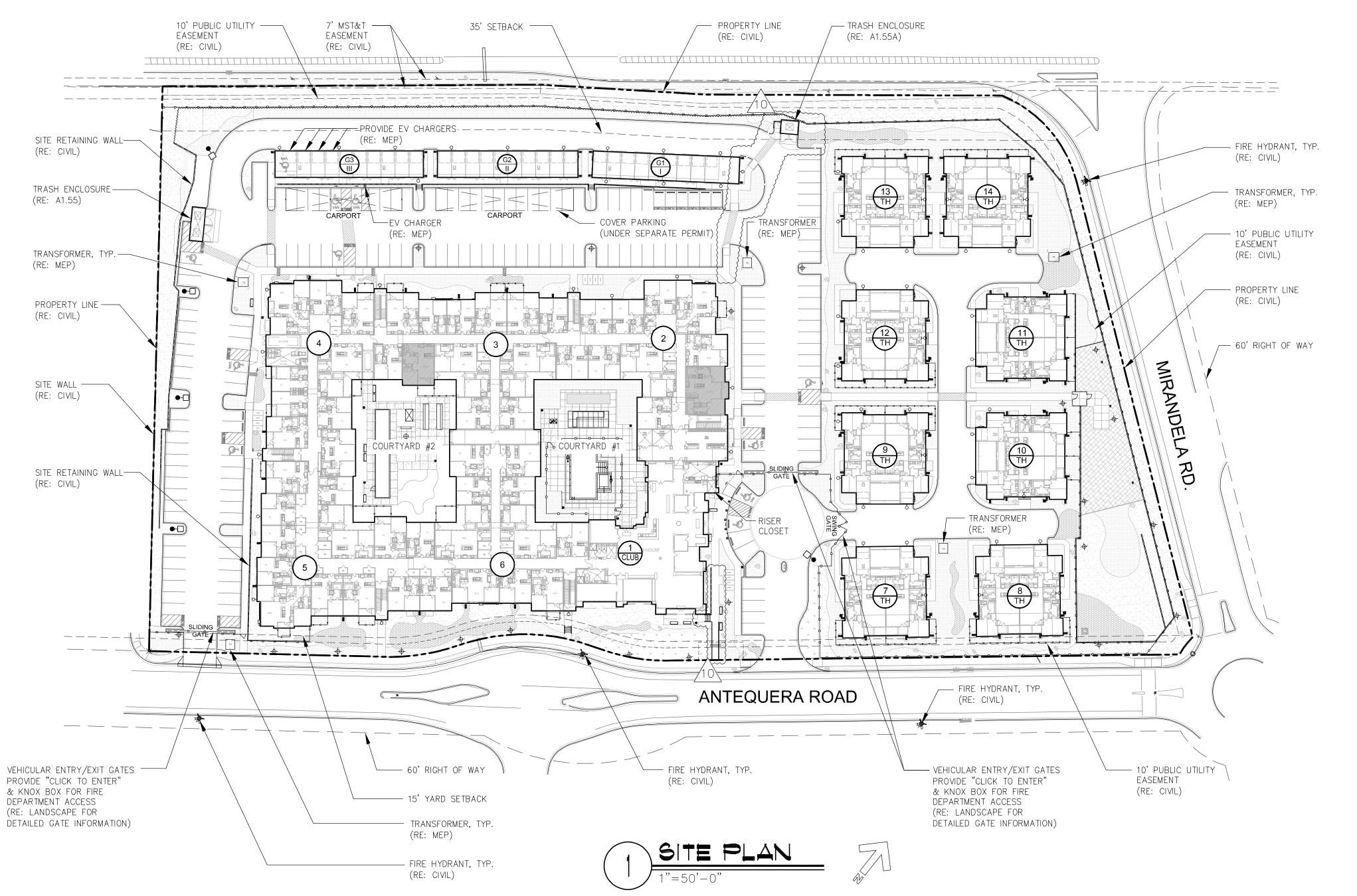
GENERAL SITE PLAN NOTES: . REFER TO CIVIL PLANS FOR ALL DIMENSIONS OF SURFACE PARKING AND PAVING, AS WELL AS FINISHED FLOOR ELEVATIONS AND SURFACE SITE DRAINAGE.
