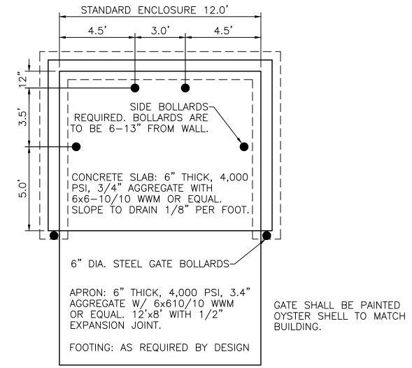
APRON REQUIRED IN FRONT OF EACH ENCLOSURE. (6" WITH REINFORCING TO WITHSTAND 57,000 LBS.)
