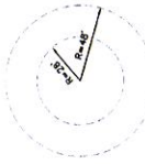
FIRE APPARATUS TURNING RADIUS 28'-0"
