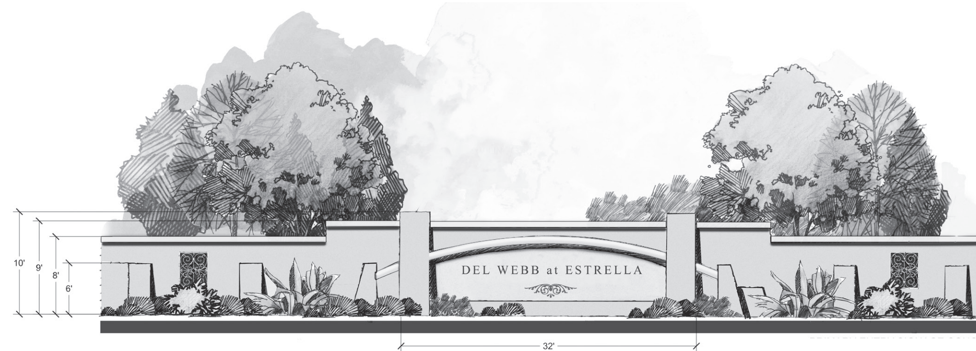
M. ILLUSTRATIVE SECONDARY COMMUNITY ENTRY - B Max. Height: 7 feet Max. Length: 15 feet Max. Sign face: 35 SF.
