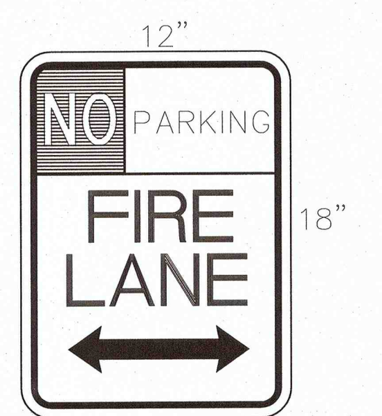
NO PARKING FIRE LANE SIGN
