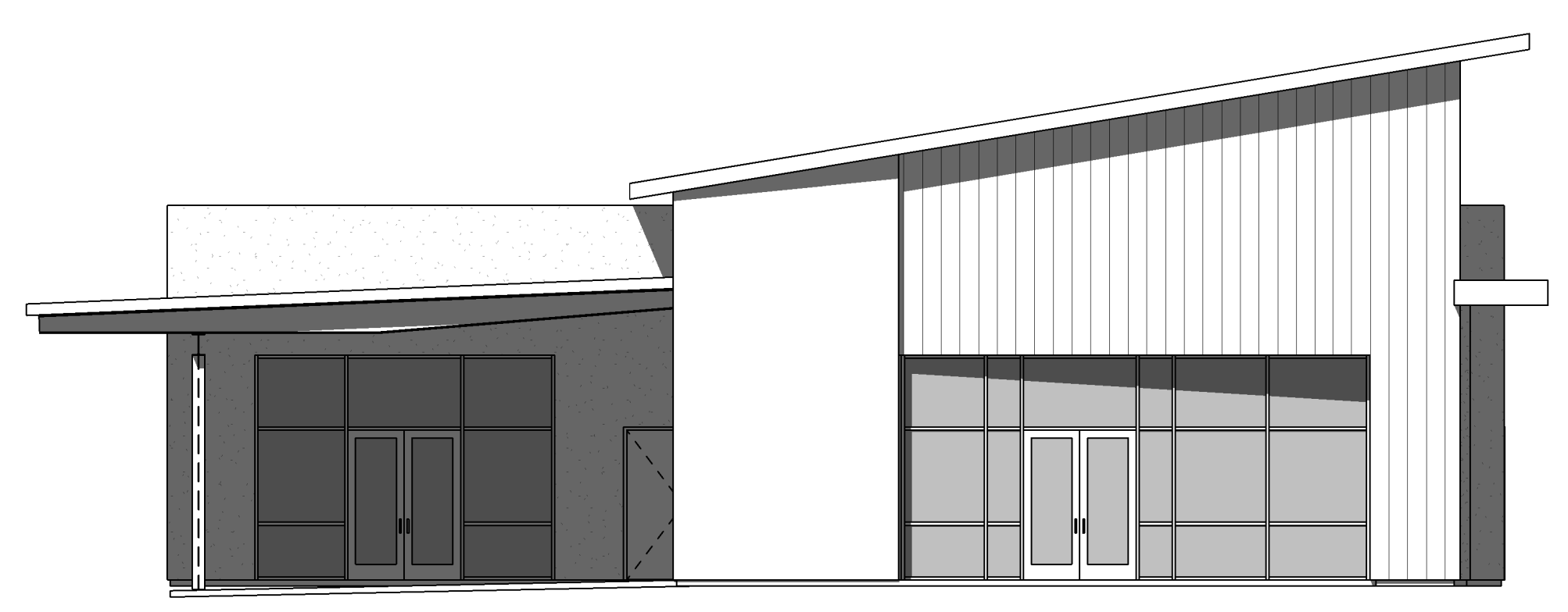
C1 SOUTH ELEVATION 1/8" = 1'-0" % EXPOSED = 55% DOES NOT ACHIEVE > 75%
