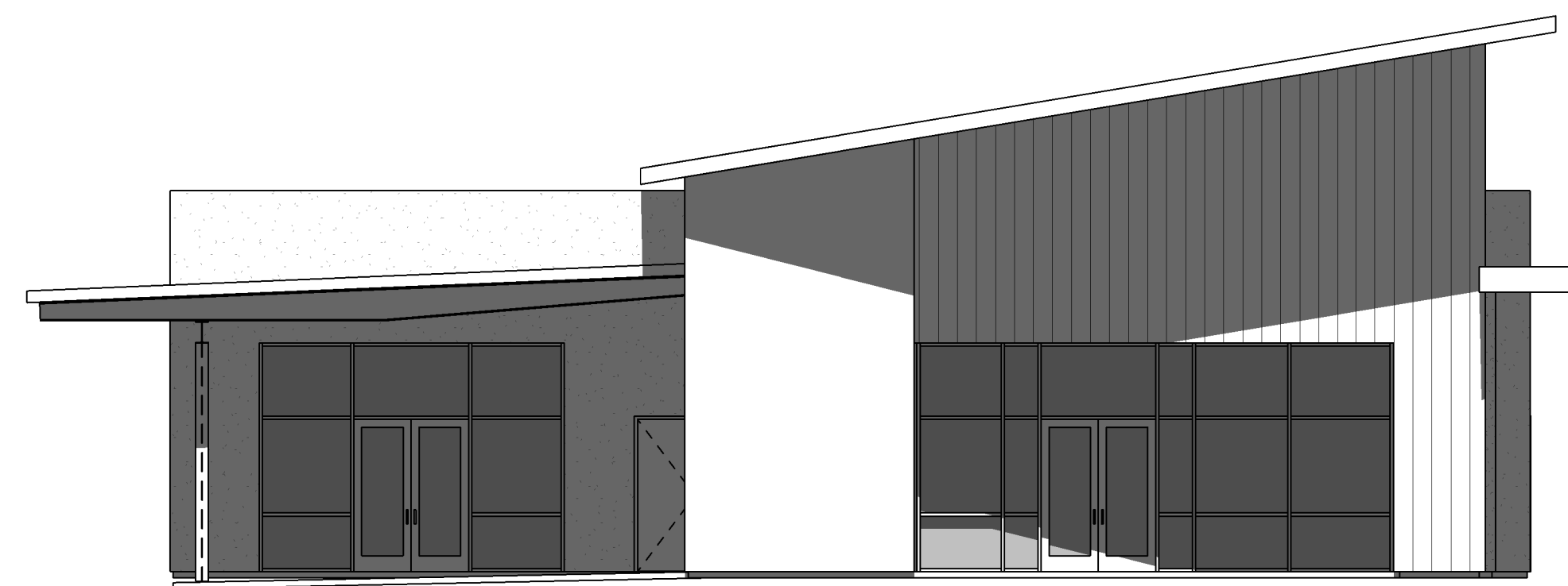
C1 SOUTH ELEVATION 1/8" = 1'-0" % SHADED = 95% ACHIEVES > 90%
